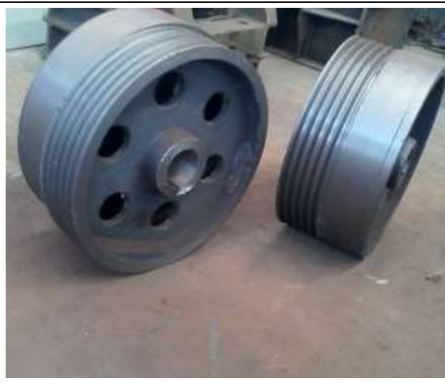
Pulley for crusher
