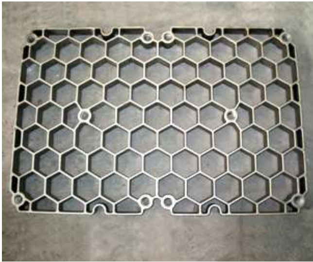
FURNACE TRAY 1300mmX700mmX50mm
